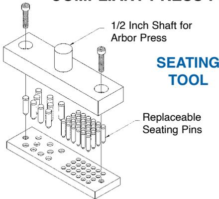
**NOTE:** Straight mount female connector seating tool shown. Right angle (90°) male and female seating tool not shown. Seating pins are not required for right angle (90°) connector seating tools.
