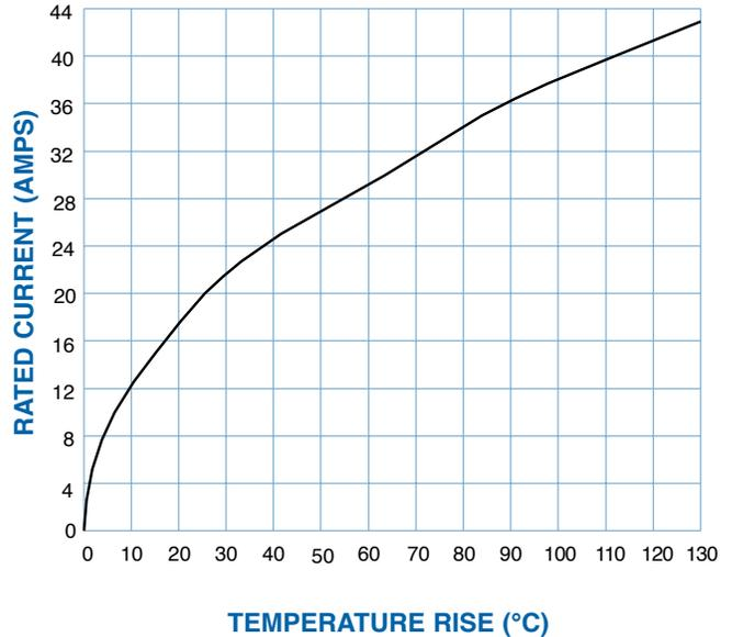
Above curve developed using MIP30M0000 and MIP30F0000 connectors with MC112N and FC112N2 contacts and 12 AWG wire. All contacts under load.
