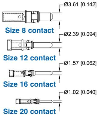
**Contact sizes and termination types may be mixed within a single connector.**
