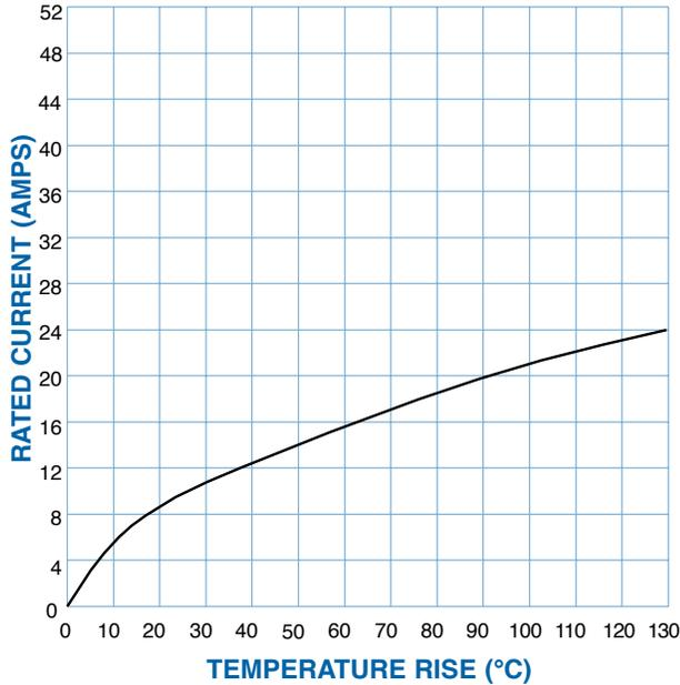
Above curve developed using IP56M400A1 and IP56F300A1 connectors and 12 AWG wire. All contacts under load.
