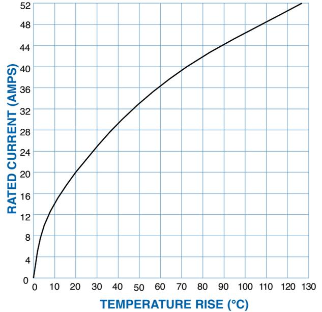
Above curve developed using a IP33W9M0000 connector with MC612N contacts and a IP33W9F0000 connector with FC612N2 contacts and 12 AWG wire on both. All contacts under load. Size 16 contact positions not filled and tested.
