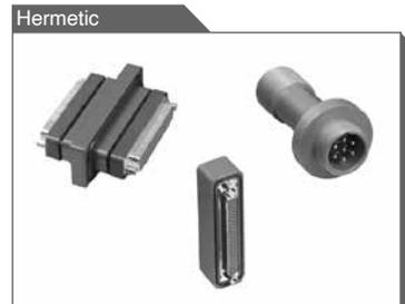
**FEATURES:** Intended for use as an electrical feedthrough in high vacuum applications • Leakage rate: 5 x 10<sup>-9</sup> mbar.l/s @ vacuum 1.5 x 10<sup>-5</sup> atm • Signal, power, coax and high voltage versions available • Connectors can be mounted on flange assembly per customer specification
