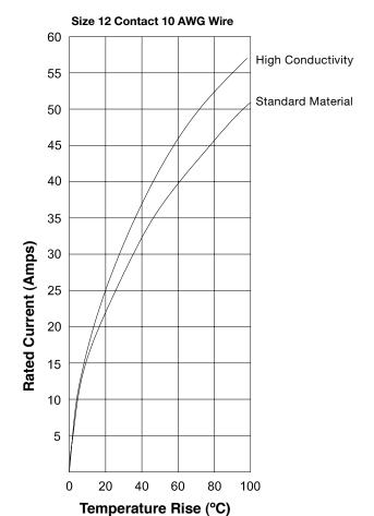
Above curves developed separately using Size 12 contact with 10AWG wire. Four (4) Size 12 contacts under load.
