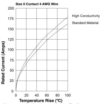
Above curves developed separately using Size 0 contact with 4 AWG wire. Four (4) Size 0 contacts under load.
