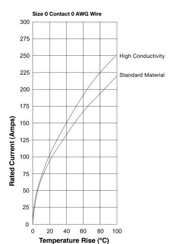
Above curves developed separately using Size 0 contact with 0 AWG wire. Four (4) Size 0 contacts under load.
