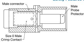
The connector was designed to pass the IEC 60950 (figure 2C) test probe which provides protection from electric shock and energy hazards.
