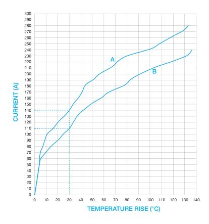
A Developed with (3) #0 high conductivity contacts with 0 AWG wire.
