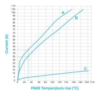
A Developed with (2) #12 high conductivity contacts with 10 AWG wire.
