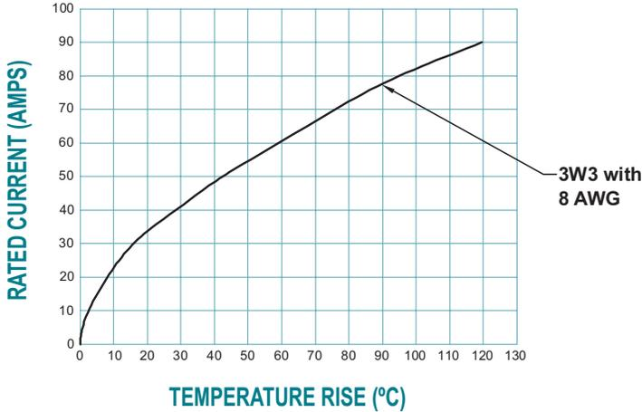
Curve developed using a mated Combination-D 3W3F loaded with size 8 crimp contacts and Combination-D 3W3M loaded with size 8 crimp contacts terminated to 8 AWG wire.
