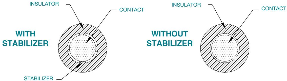
SCBM size 8 male contacts are removed toward the rear after utilizing front release tooling. Space must be provided between the contact and the connector molding so the tooling can slide over the mating portion of the contact. This fact allows the contact to float.
