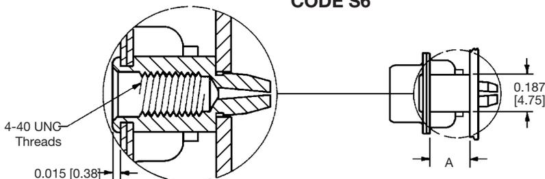
Printed board mounting hole to be 0.123 [3.12] Ø ±0.003 for use with push-on fastener.
