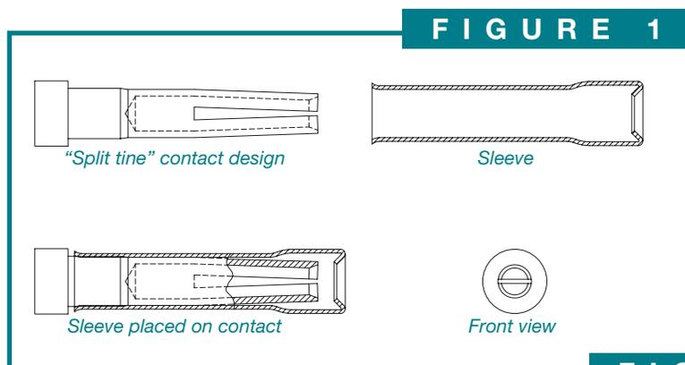
The most common **closed entry design** utilized by connector manufacturers is a split tine and sleeve concept. **See figure 1.** With this design, both the mechanical forces and electrical interface are provided only at the tip of the female contact.
