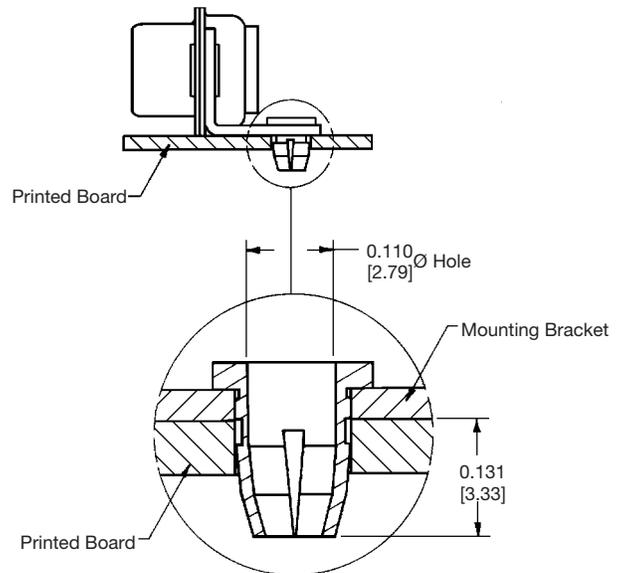
Printed board mounting hole to be 0.123 [3.12] Ø ±0.003 for use with push-on fastener.
