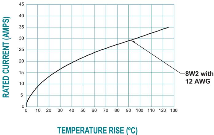
Curve developed using a mated Combination-D 8W2M loaded with size 8 crimp contacts and Combination-D 8W2S loaded with size 8 crimp contacts terminated to 12 AWG wire.
