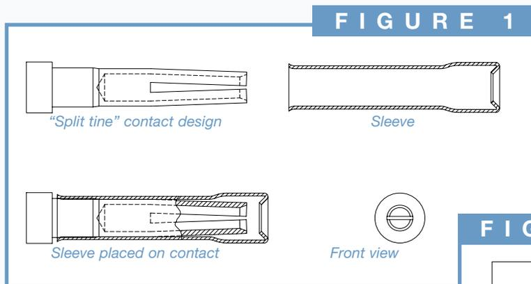
The most common **closed entry design** utilized by connector manufacturers is a split tine and sleeve concept. **See figure 1.** With this design, both the mechanical forces and
