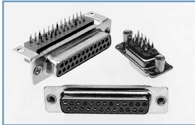
PCD series connectors are quality connectors with compliant terminations. The low press-in force required to install the contacts into the board eliminates printed board pressure-warp and twisting stresses which can result in expensive repair or replacement of printed boards and back panels.
