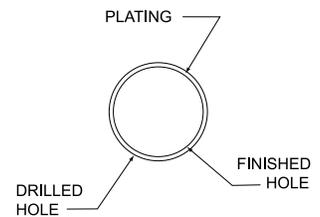
**COMPLIANT PRESS-FIT TERMINATION CONTACT HOLE**
