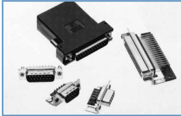
Melo-D series connectors are professional quality connectors recommended for use in sheltered, non-corrosive indoor or outdoor environments having normal ventilation, but without temperature or humidity controls. These fixed contact connectors meet the dimensional and performance requirements of IEC 60807-2, Performance Level Two.
