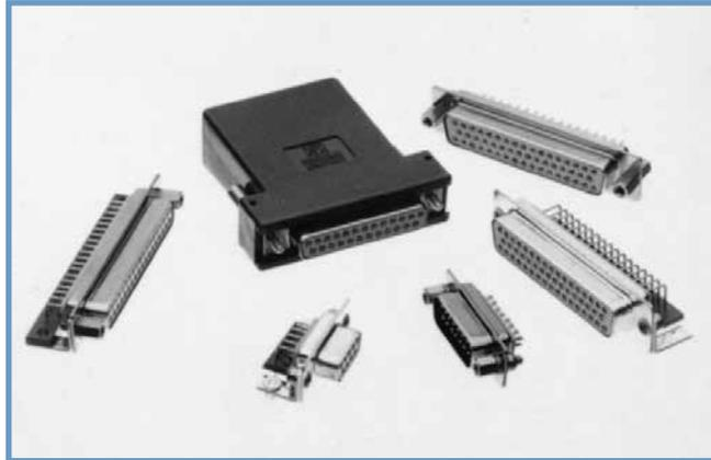
Harmo-D series connectors are military quality connectors designed for use in sheltered, mildly corrosive environments having a wide range of temperature, pressure and humidity changes. Applicable fixed contact connectors are qualified to MIL-DTL-24308 (see page 82 for more information) and meet the performance requirements of IEC 60807-2, Performance Level One.
