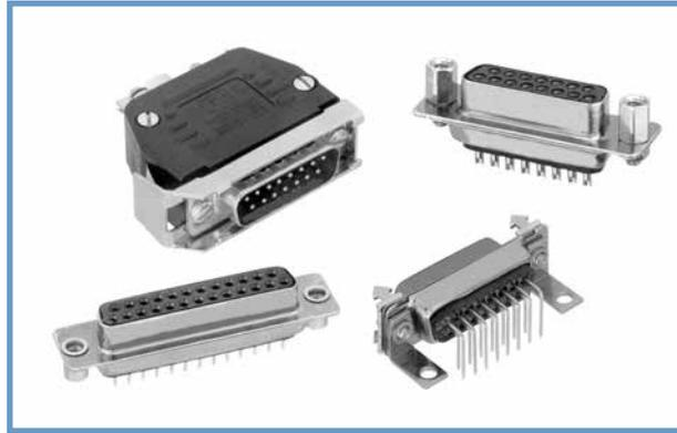
Euro-D series connectors are professional quality connectors recommended for use in sheltered, non-corrosive indoor or outdoor environments having normal ventilation, but without temperature or humidity controls. These fixed contact connectors meet the dimensional and performance requirements of IEC 60807-2, Performance Level Two.
