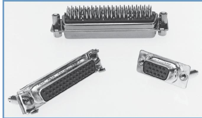
PCDD series connectors are quality connectors with compliant terminations. The low press-in force required to install the contacts into the board eliminates printed board pressure-warp and twisting stresses which can result in expensive repair or replacement of printed boards and back panels.
