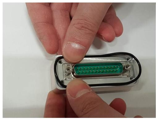
Continue to insert the O-ring by pressing along the perimeter of the O-ring inserting into the groove.
