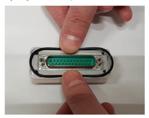
Press the O-ring into the groove on one side of the connector.
