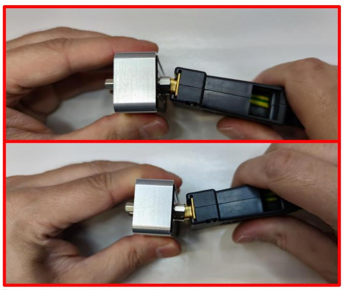
The angle is slightly exaggerated in the photos to clearly illustrate the meaning of the up and down movement during the plugging and unplugging process.
