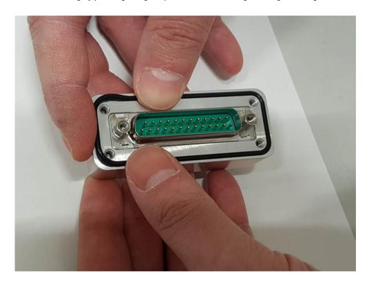
Check to make sure the O-ring is fully inserted into the groove with no bubbling of any kind.
