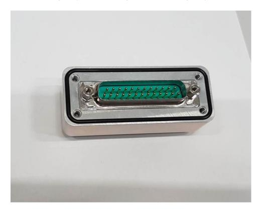
If the O-ring contains bubbles as shown below, remove the O-ring and start the assembly process over.
