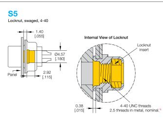
\*1 Non-removable threaded hardware is built and inspected to 5in/lbs or 80 in/oz torque.
