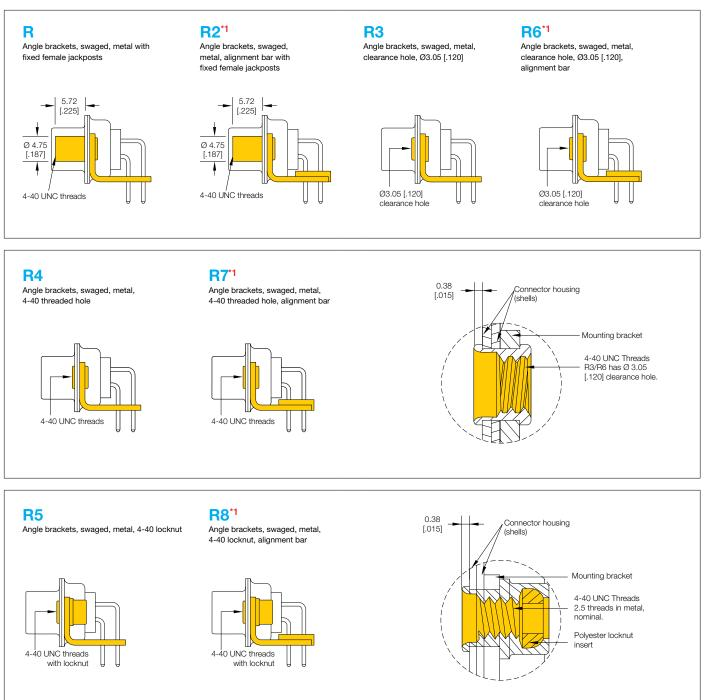
\*1 Contact alignment bar is supplied with R2, R6, R7 and R8 options only.
