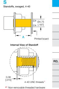
Non-removable threaded hardware is built and inspected to 0.56 Nm [5in/lbs] or 80 in/oz torque.
