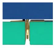
Press-fit connectors therefore remain a popular choice for PCB designers. To provide a modern solution that will provide the benefits of press-fit termination without the drawbacks, Positronic has created a solution using contacts with compliant tails. Named "Omega" after the Greek letter that they resemble, their flexibility ensures the same stable mechanical and electrical joint without the damage to the through-hole plating.
