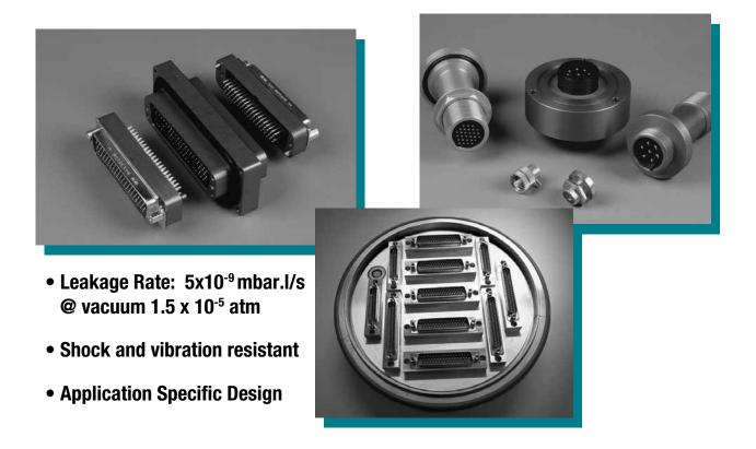
Positronic Industries can supply hermetic connector assemblies for use in vacuum applications. All Positronic hermetic connectors are designed to act as feedthroughs through the bulkhead/chamber wall. Typically both sides of the connector have mating faces, but certain contact terminations are also available per customer requirement. Typical configurations include:
